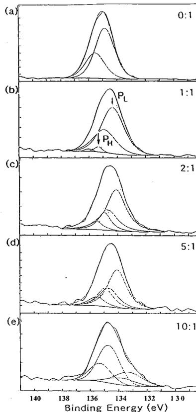
FIG. 3. Core level spectra of P 2p observed for the Ce(IV)/DPP mixtures, with the molar ratios of (a) 0:1, (b) 1:1, (c) 2:1, (d) 5:1, and (e) 10:1.  $P_H$  and  $P_L$  correspond to the doublet peaks of higher and lower binding energies.
